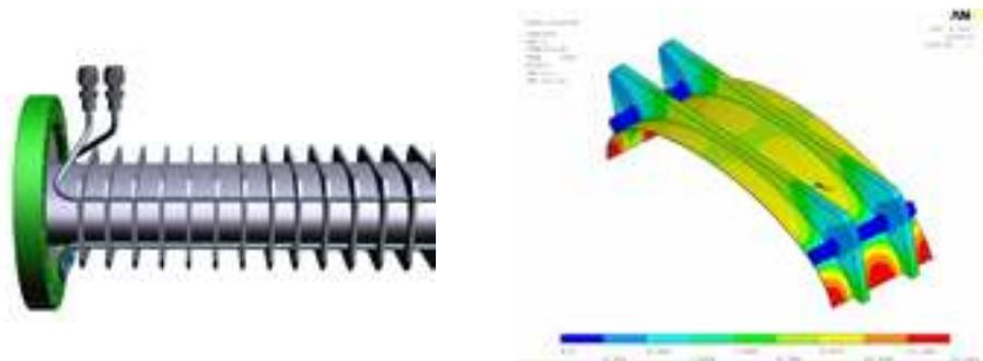
**Figure 2 - Left: Schematic drawing of dipole chamber with cooling tubes and ribs. The length of the chamber is 3.35 m with an aperture of  $120 \times 60 \text{ mm}^2$  and a bending angle of  $3.33^{\circ}$ . Right: ANSYS calculations of the temperature distribution of the dipole chamber.**
