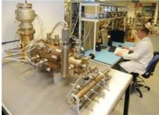
Figure 4 - New vacuum gauge calibration service.
