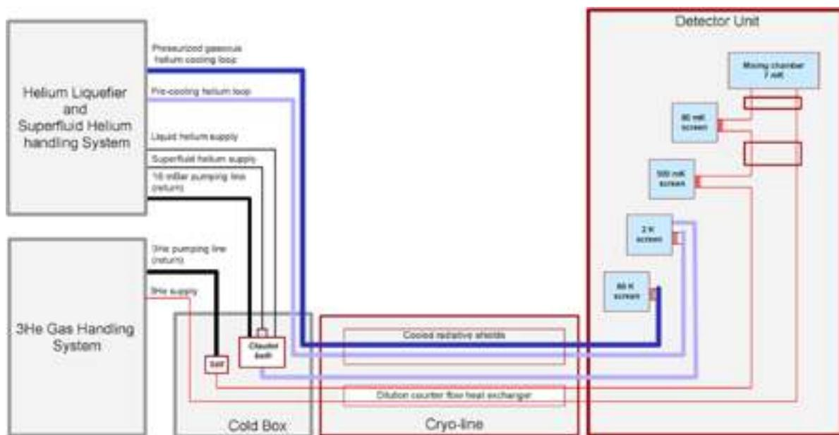
Figure 2 - Schematic of the EURECA cooling system.
