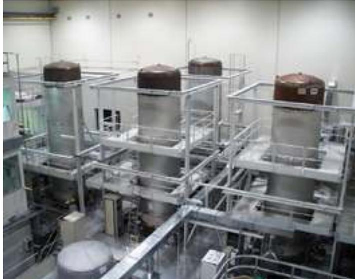
**Figure 3 - The Virgo towers; 11 m high, 2.0 m diameter.**
