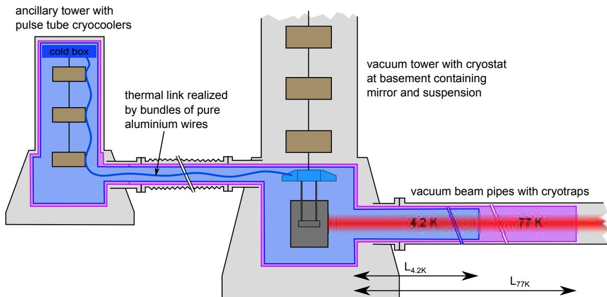
**Figure 5 - Schematic of vacuum towers (containing optical components in cryostats) at the end of a beam pipe. The thermal load from the warm (ambient temperature) beam pipes is reduced by up to 60 m long cryotrap, which are attached inside the vacuum tubes in front of the mirrors.**
