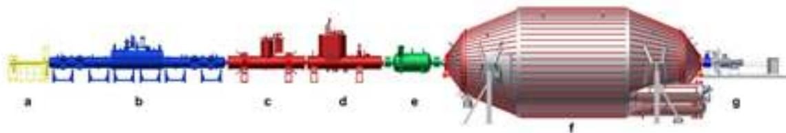
**Figure 1** - Components of the KATRIN experiment are a) the calibration and monitoring section, b) windowless gaseous tritium source (WGTS), c) differential pumping section (DPS) with turbo-molecular pumps, d) cryogenic pumping section (CPS), e) pre-spectrometer, f) main spectrometer and g) the detector system. The setup has a total length of about 70 m.
