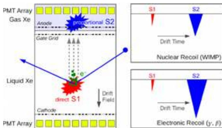
Figure 1 - The principle of a typical two-phase TPC.
