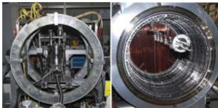
**Figure 2 - Left: Helmholtz coils and TMP for the measurement of the rotor heating through eddy currents. Right: One getter pump in the main spectrometers (1000 m of SAES St707 NEG strips) with a pumping speed of 340 000 l/s and a LN<sub>2</sub> cooled cryo-baffle for radon capture. The baffle reduces the effective pumping speed to 150 000l/s.**
