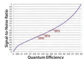
Figure 1: Development of the quantum efficiency and resulting signal-to-noise ratio of PMTs. Note that in the time between the 1960s until 2005 it was believed that this technology cannot be further advanced.
