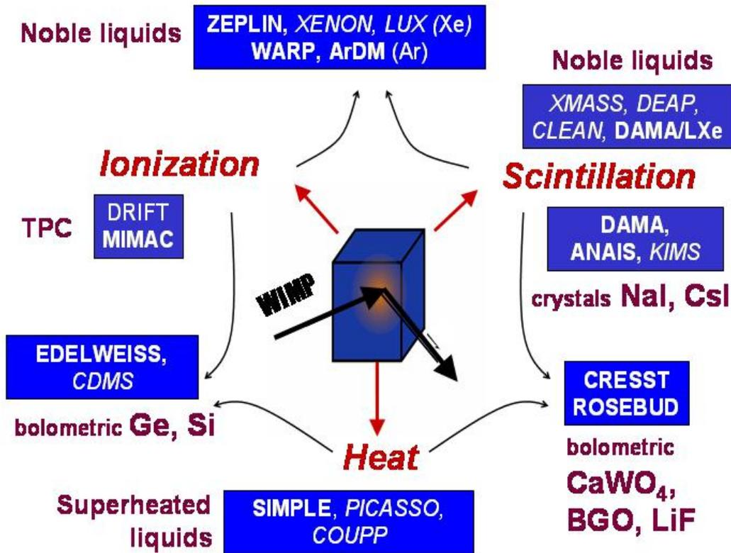
**Figure 3.2:** Methods and present experiments/prototypes for direct WIMP detection. Experiments with a clear European lead role are in bold face, experiments without or with small European participation are in italics. DRIFT (Boulby mine) has similar American and European contributions. Superheated liquid methods are here assigned to ionization to avoid confusion with phonon detection in bolometric detectors.
