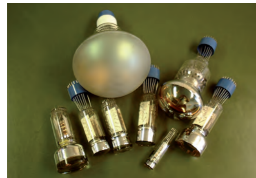
Low temperature pmts for operation to -196 deg. C
