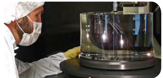
ZYGO provided approximately fifty ~340 mm diameter optics of 0.3 nm RMS quality.
