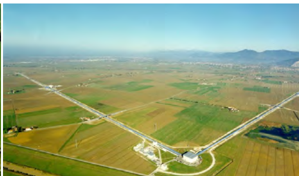
Aerial View of the Virgo detector (Cascina, Pisa, Italy). Arms of 3 km long are well visible.
