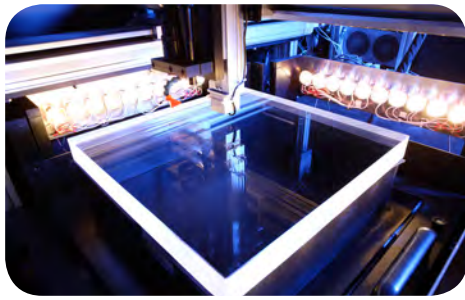
Bubble and inclusion inspection detection limit 10 µm Ø
