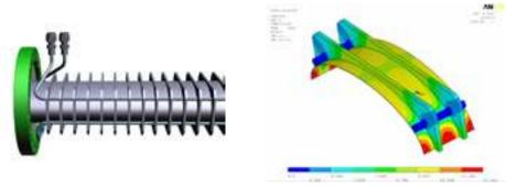
Figure 2 - Left: Schematic drawing of dipole chamber with cooling tubes and ribs. The length of the chamber is 3.35 m with an aperture of 120x60 mm<sup>2</sup> and a bending angle of 3.33°. Right: ANSYS calculations of the temperature distribution of the dipole chamber.
