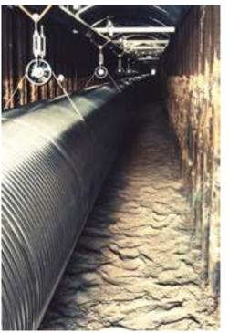
Figure 2 - The GEO600 vacuum pipe; 600 m long, 0.6 m diameter, 0.8 mm thick corrugated wall of 316L stainless steel.
