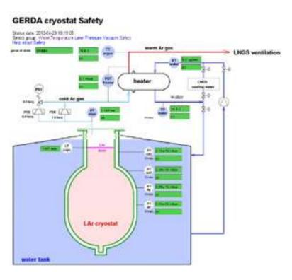
Figure 3 - Safety status of the GERDA experiment at 18:19:05 on April 23, 2012. The safety relevant parameters are cryostat pressure, fill level, residual and total vacuum pressures, the flow rate and the temperature of the LNGS cooling water, as well as the temperature of the argon exhaust gas. The flow rate of the argon exhaust gas is deduced from a measurement of the differential pressure at the input and output of the heater.
