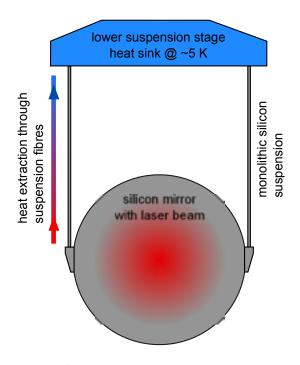
Figure 4-Schematic of the heat extraction from a mirror substrate to a heat sink at about 5 K. To attenuate seismic disturbances the mirror is suspended by means of thin silicon fibres. These fibres also allow the extraction of heat which is due to optical absorption of laser light and thermal radiation.
