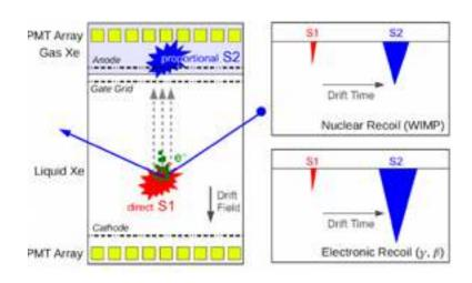
Figure 1 - The principle of a typical two-phase TPC.
