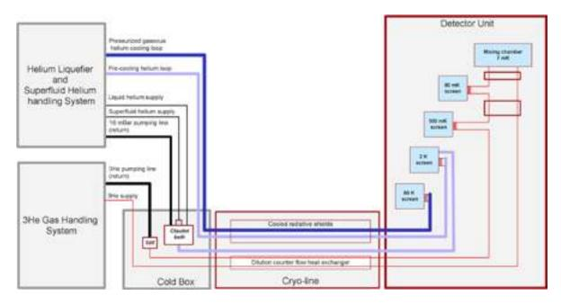
Figure 2 - Schematic of the EURECA cooling system.
