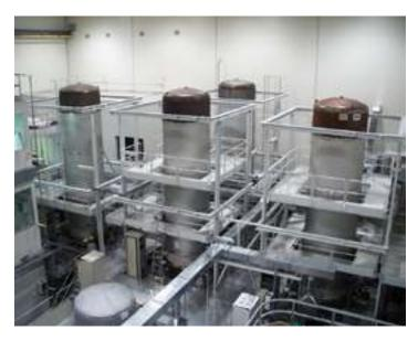
Figure 3 - The Virgo towers; 11 m high, 2.0 m diameter.
