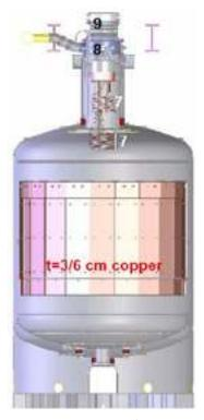
Figure 2 - Characteristics of the GERDA cryostat, and its cross section with active cooling system (7), manifold (8) and the interface (9) to the lock consisting of a bellow and a DN630 shutter. The tiny red rectangles show the locations of the Torlon support and alignment pads of the inner vessel. The bellow in the neck of the inner vessel for compensating thermal shrinkage is barely visible. Detailed drawings are available at [5].
