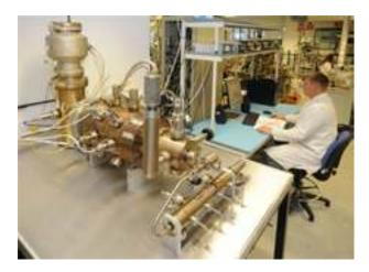
Figure 4 - New vacuum gauge calibration service.
