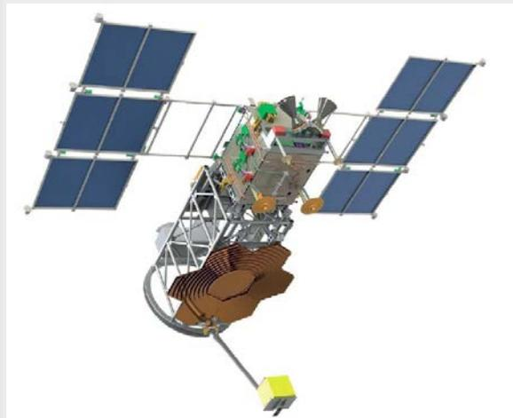
The primary instrument is the TUS (Tracking Ultraviolet Setup) instrument, which employs a large Fresnel-type mirror-concentrator to collect UV radiation over a two-square metre area and feeding it to a camera consisting of 256 photomultiplier tubes placed in the focal plane of the concentrator.
